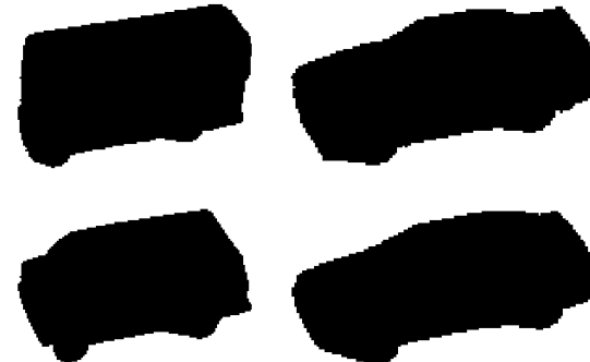
Fig. 9.2: Vehicle silhouettes prior to high level feature extraction. These are clockwise from top left: Double decker bus, Opel Manta 400, Saab 9000 and Chevrolet van.
